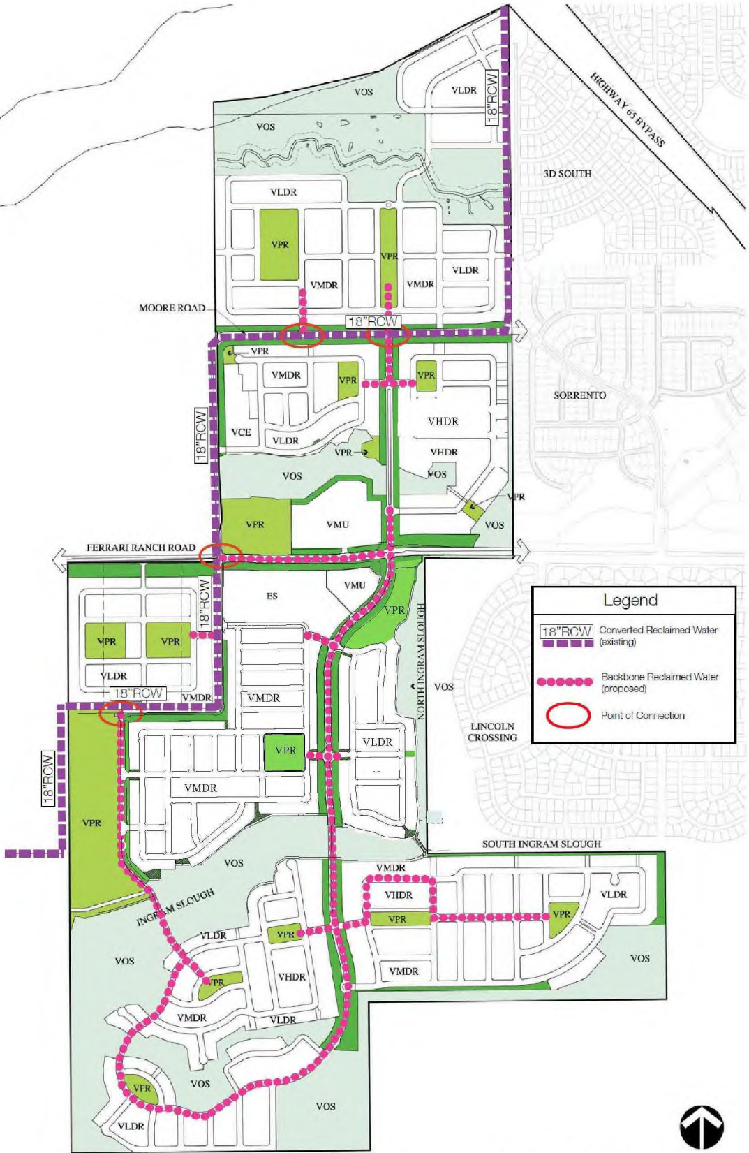
Figure 7-3: Backbone Reclaimed Water Distribution System
