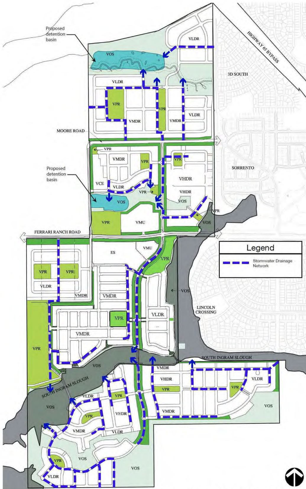
Figure 7-6: Backbone Drainage System
